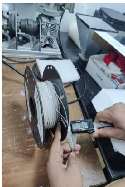
Figure 3: Digital caliper measurement of HDPE:UHMWPE (70:30) extruded filament showing a diameter of approximately 1.65 mm.
