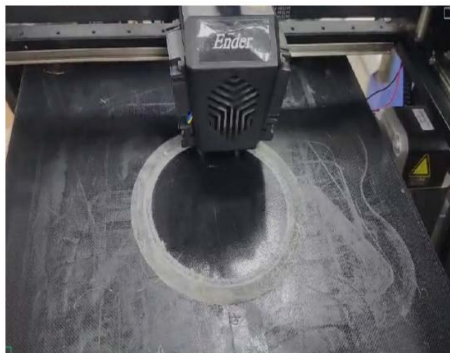
Figure 7: 3D printed part using HDPE:UHMWPE (70:30) blend filament showing poor surface finish and inconsistent deposition.
