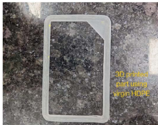
Figure 6: 3D printed part using neat HDPE (HD50MA180) filament showing excellent surface finish and dimensional accuracy.
