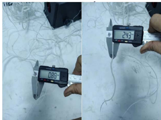
Figure 4: Extruded filament of HDPE:UHMWPE:PEG (60:40:10) showing severe non-uniformity and curling.
