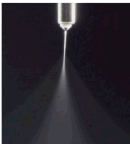
Figure 1: Taylor cone generated during an electrospraying process. Taken from [17].
