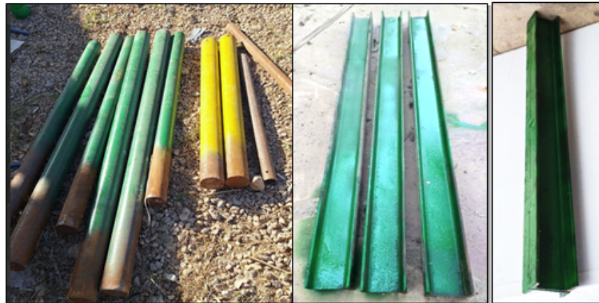
Figure 2: Model piles used in the experimental program, including closed-ended pipe piles and fabricated H-section piles designed with equivalent cross-sectional areas.
