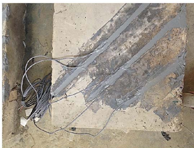
Figure 4: Near-surface mounted (NSM) polymer-based CFRP bars after complete filling of grooves with epoxy adhesive. The epoxy encapsulation ensures effective polymer-concrete bonding, protection of CFRP bars, and reliable stress transfer within the shear zone of the deep beam specimen.
