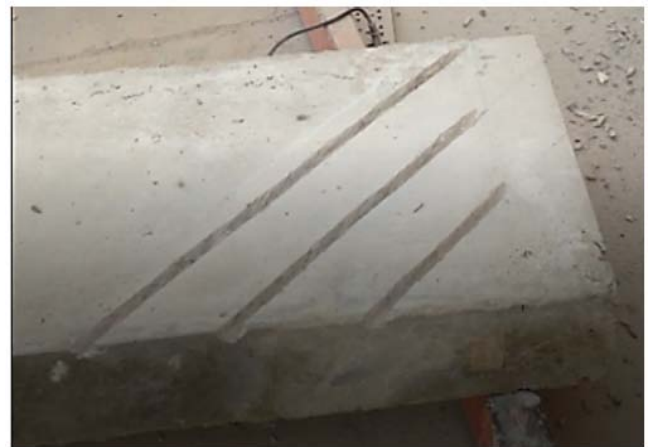
Figure 2: Preparation of near-surface mounting (NSM) grooves cut into the concrete cover of a deep beam specimen prior to installation of polymer-based CFRP bars. The inclined grooves were formed to accommodate CFRP bar placement and ensure effective bonding with the epoxy adhesive.
